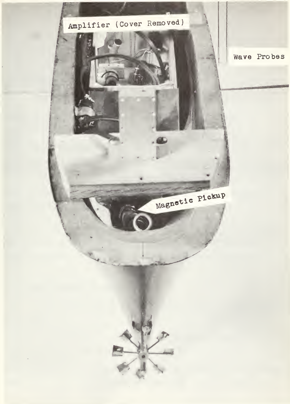
Ship Model with Instrumentation Installed
